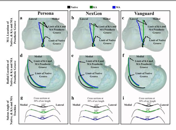
**Fig. 8** Schematic of a representative knee shows tracings of the M–L and radial locations of the groove and sulcus angle of the native trochlea (black), and the KA (green) and MA (blue) positioned prosthetic trochlea of the Persona, NexGen, and Vanguard femoral components. In general, the M–L and radial locations of the KA prosthetic trochlea are closer to native than those of MA [18]. The M–L
