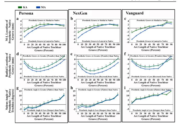
**Fig. 7** Series of graphs showing the differences between the prosthetic and native for KA (green lines) and MA (blue lines) in the medial–lateral and radial locations of the groove and sulcus angle of the trochlea at intervals from 0 to 100% of normalized arc length of the native trochlear groove for three femoral component designs. The
